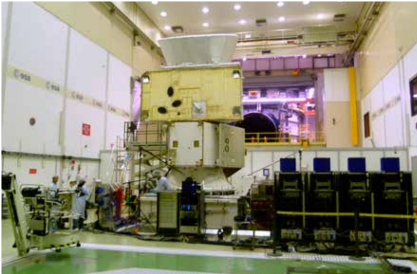
Preparing BepiColombo for vibration testing, ensuring the spacecraft will survive the brutally jolting start of its journey to Mercury atop the Ariane 5 launch vehicle.
