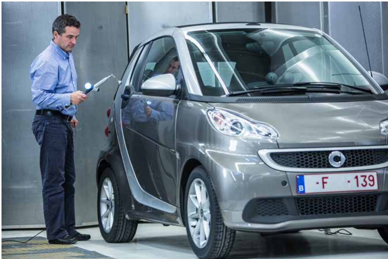
Measuring transmission loss on an automotive car door.
