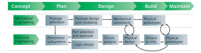
The process generally begins with the electrical engineer defining the overall system and then segmenting it into various electrical subsystems. The logical performance and physical characteristics of each subsystem has constraints and dependencies associated with the rest of the product, such as with the software to be embedded, the mechanical enclosure and the electrical interconnect required to tie the various subsystems together.
