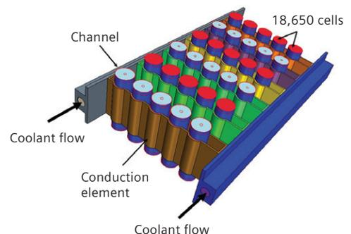
Figure 1: Geometry of the pack and the thermal management system.
