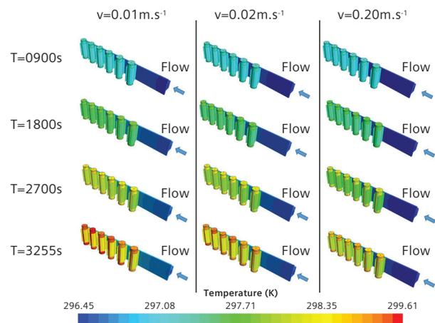
Figure 2: The temperature rise in the first set of series cells in the pack is a function of the .9 Celsius (°C) discharge rate and contact resistance of .0025 (m<sup>2</sup>.°K)/W.
