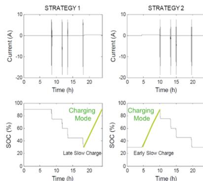
Unlike classic usage in which the PHEV Li-ion battery is recharged at the end of the daily mission, “just-in-time” charging allows for reducing battery degradation phenomena.
