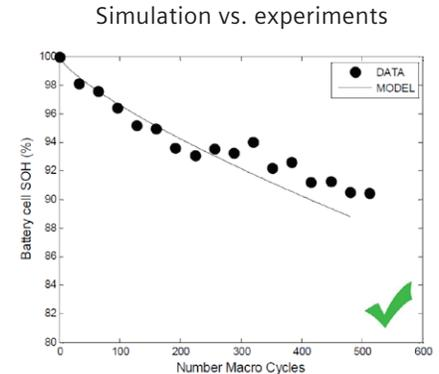
The PHEV battery aging model takes into account daily driving, parking and recharge cycles.
