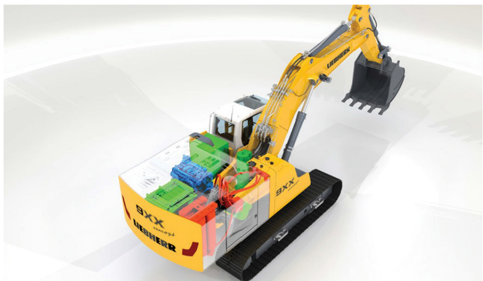
R 9XX concept, a Liebherr electro-hydraulic hybrid crawler excavator, demonstrates the energy recuperation technology. It has a fully integrated mechatronics system, including hydraulic, electric and energy management components.
