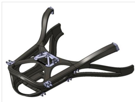
Design and optimization of composite vehicle frames performed by IPM students using NX.
