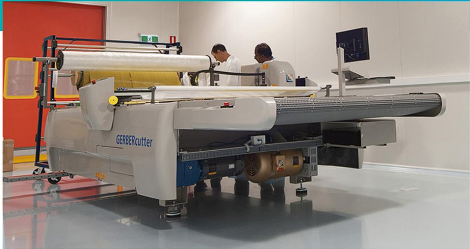
*Fibersim exports flat patterns directly to Quickstep’s cutting machine (shown above). This process is completely digitized and, as a result, increases the efficiency of the production process and improves the overall quality of the composite parts.*
