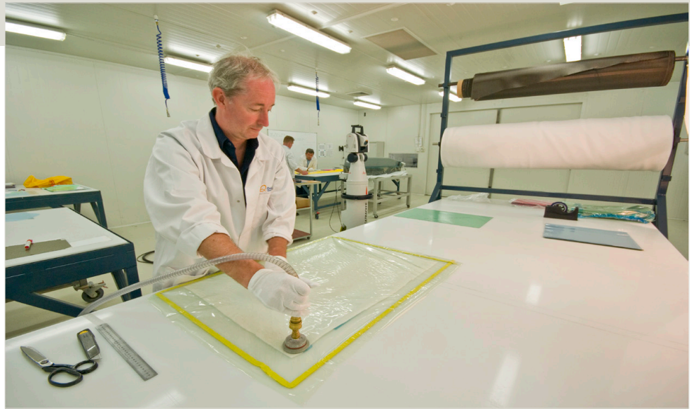
Shown is a stage in the layup process at Quickstep. Fibersim creates the flat pattern shape for the cutting machine to cut out. This ensures that the flat patterns can be accurately and efficiently laid up to create the composite part.
