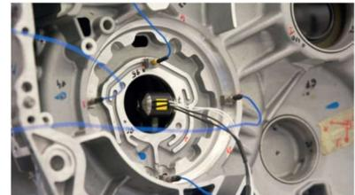
Additionally, the data acquisition can be executed by only one operator. The miniature shaker can be used with Simcenter Testlab software Spectral Testing or MIMO FRF testing together with the Simcenter Qsources measurement amplifier. The integrated transducers are IEPE type sensors and are compatible with Simcenter SCADAS hardware input modules.
