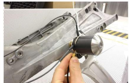
without external support or the need for alignment. Thanks to the patented internal suspension, the inert mass is dynamically decoupled from the test object and the force is always aligned along the internal stinger axis. This significantly improves the efficiency of testing by eliminating the support and alignment work associated with conventional shaker testing. Additionally, you only need one operator to execute data acquisition.
