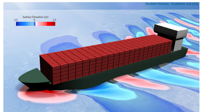
Volume of fluid (VOF) simulation of the waves around a cargo vessel.
