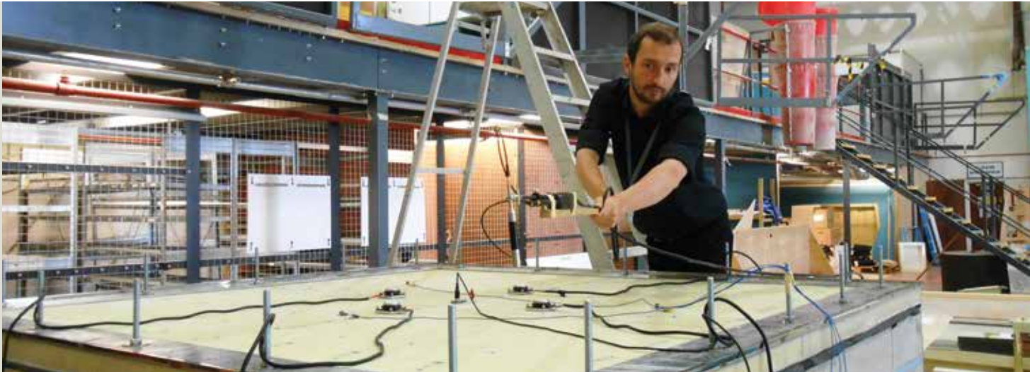
The Panel testing facility or PTF in factory unit in Plymouth, UK is made of more than 3.5 tons of concrete. It is a mini-version of a two-chamber anechoic/reverb setup.
