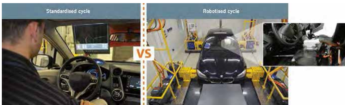
FIGURE 1 Standardised cycle measurements for regulation versus robotised cycle measurements for detailed analysis (  Siemens)
