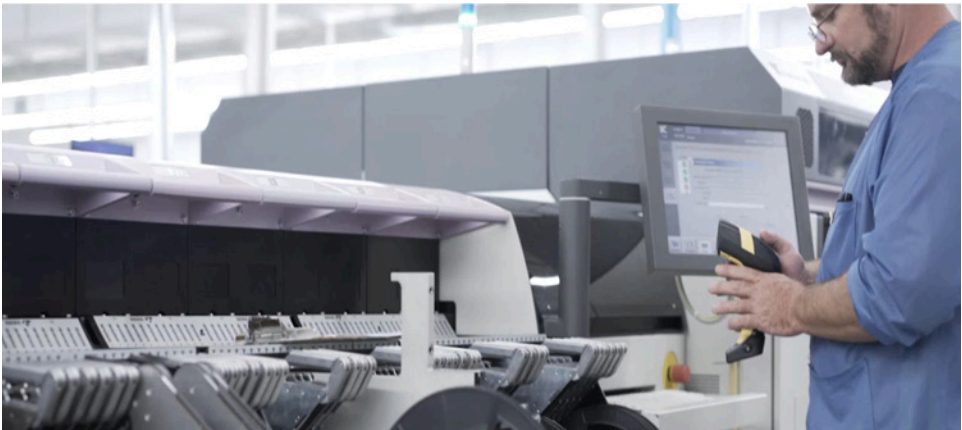
Figure 7.3: Hand scanners, in addition to in-line sensors, can be part of real-time smart manufacturing.
