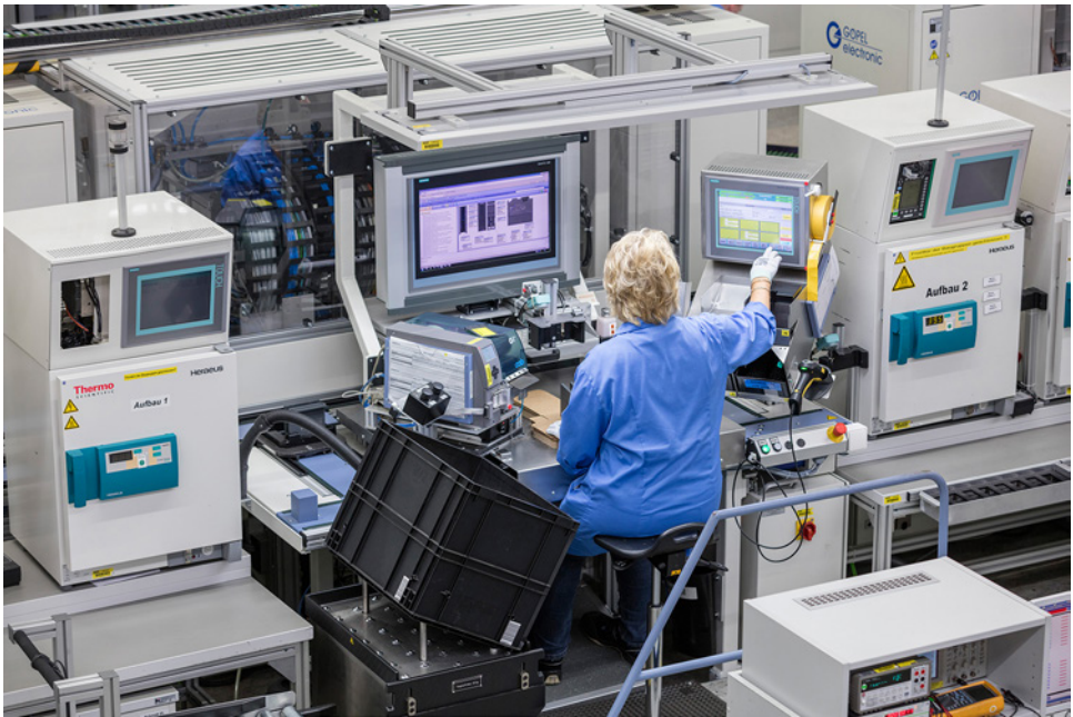
Figure 8.9: A portion of the Siemens Amberg automated plant producing programmable logic controllers (PLCs).
