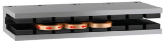
Figure 6: An example of a permanent magnet assisted switched reluctance machine using three actuator systems.
