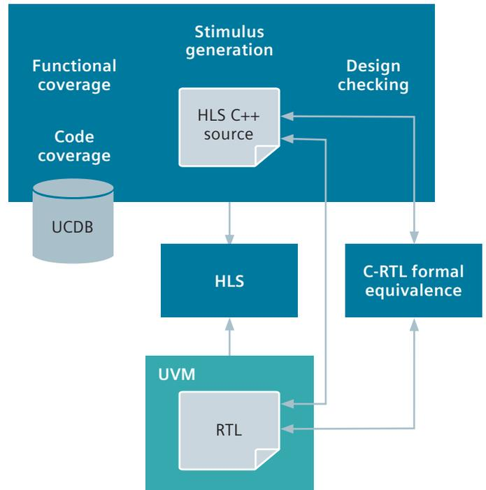
Figure 2: Advanced HLS flows HLS can perform C-to-RTL verification to remove bugs and errors before committing to RTL.
