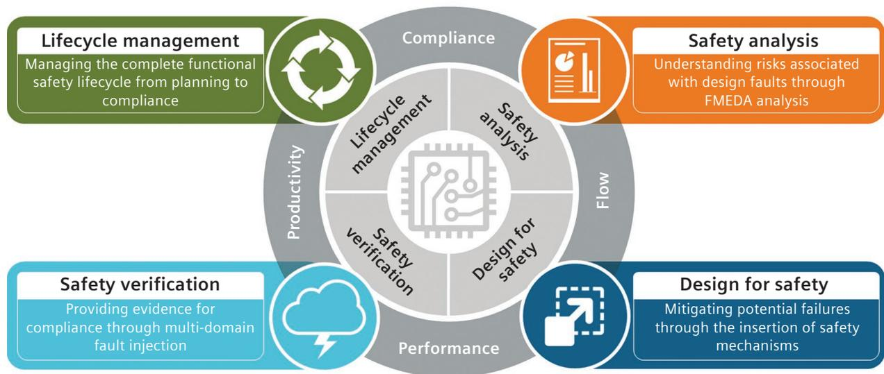
Figure 4: The four key processes in functional safety include lifecycle management, safety analysis, safety verification and design for safety.
