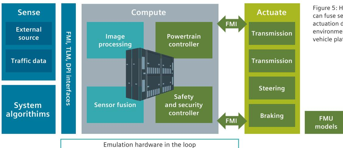
Figure 5: Hardware emulation can fuse sensor, compute and actuation data to create a testing environment for autonomous vehicle platforms.
