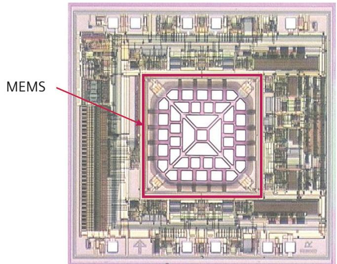
Figure 6: A MEMS device integrated on a CMOS IC.
