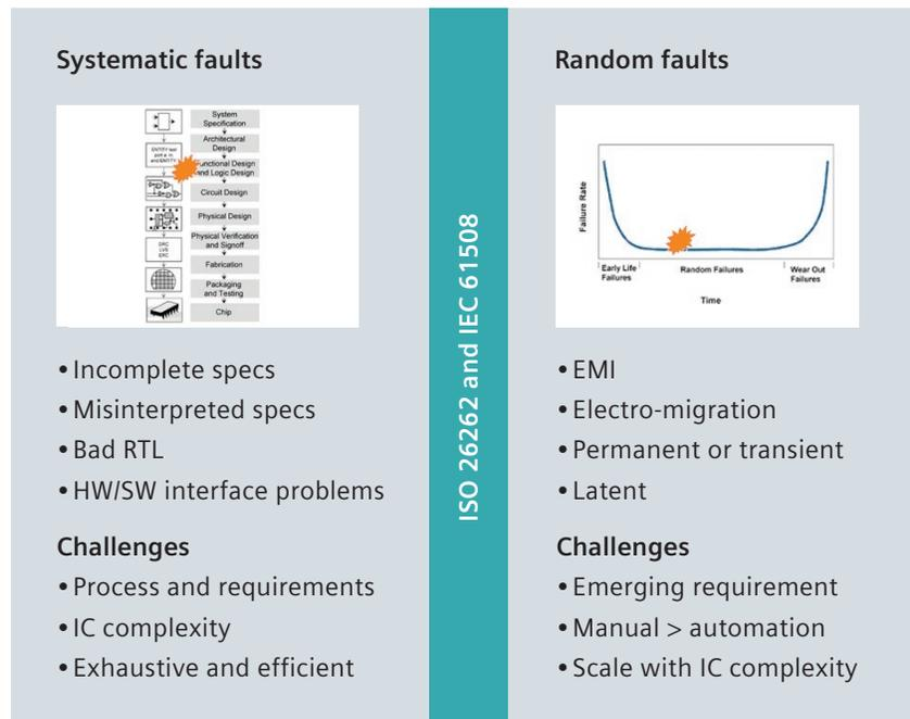
Figure 3: ISO 26262 requires that electronics are tested for systematic and random faults.
