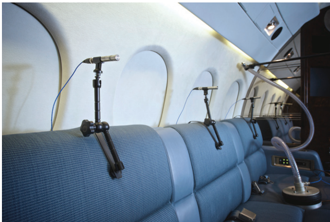
The transfer path analysis technique helps find the root cause of noise and vibration issues (image courtesy of Belgian Defense Forces).
