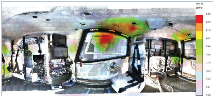
A spherical array allows rapid sound source localization throughout the aircraft cabin.
