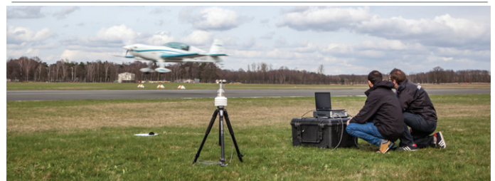
Impact of electric propulsion estimated with a flyover noise measurement setup.
