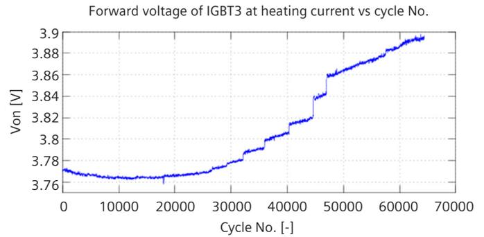
Figure 10: Forward voltage of IGBT3 at heating current level as function of applied power cycles.
