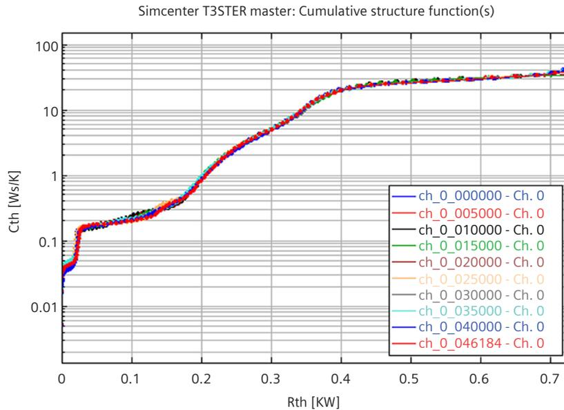
Figure 8: Change of the structure function of IGBT1 during the power cycling.
