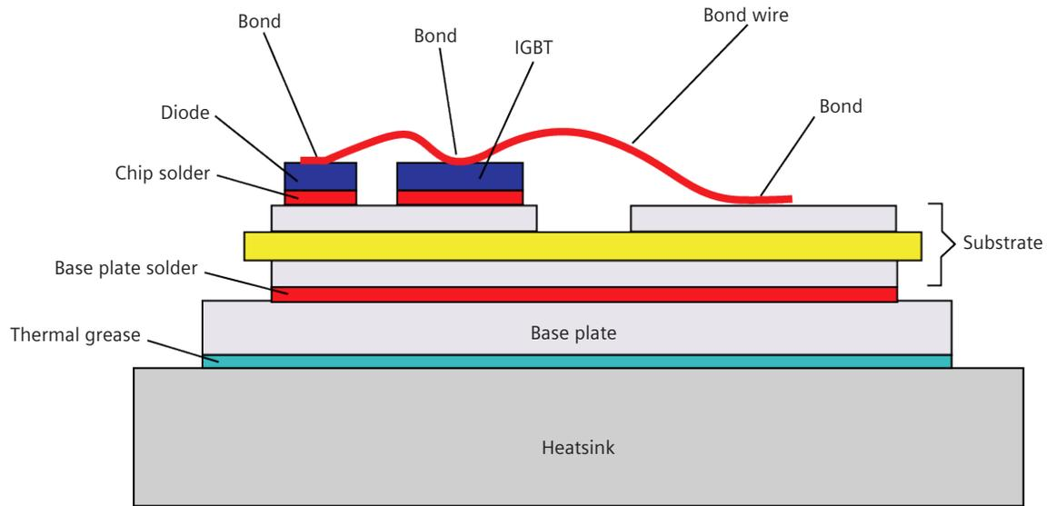
Figure 6: Cross-section of a typical IGBT module.
