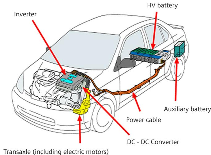
Figure 2: Power electronics components inside a HEV.
