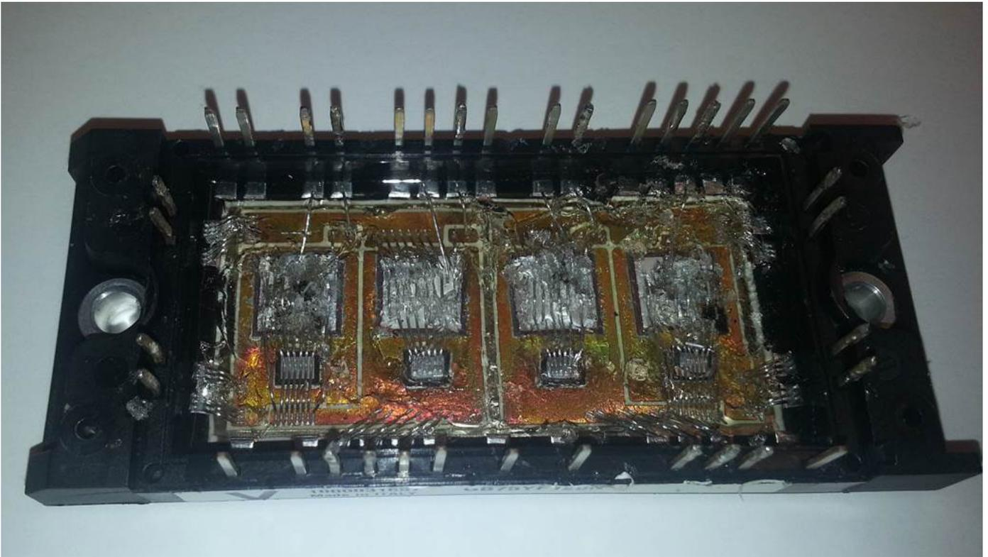
Figure 3: IGBT module after experiencing thermal damage.
