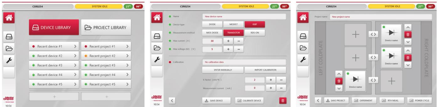
Figure 5: The Simcenter POWERTESTER 1500A touch-screen interface (left to right): main screen, device creation, and placing devices on the cold plate.
