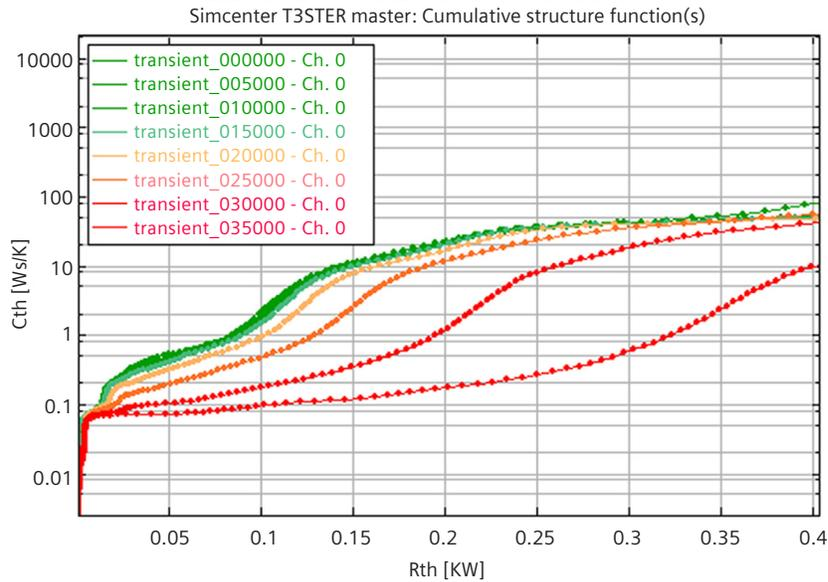
Figure 7: Structure functions of sample 0 corresponding to control measurements at various time points.
