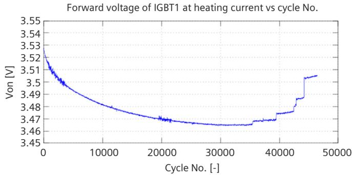
Figure 9: Forward voltage of IGBT1 at heating current level as a function of applied power cycles.
