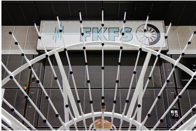
Use of customized acoustic arrays for wind tunnel sound source localization. Example of one of the acoustic arrays.
