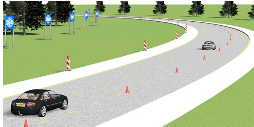
Figure 8: ACC use case: object selection in a curve [ISO 15622].
