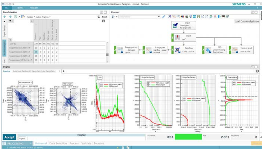
Figure 3: Comparing two time signals with embedded load analysis in Simcenter Testlab.
