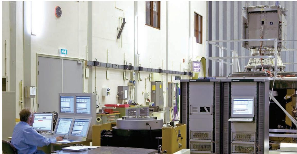
Simcenter Testlab Environmental provides you with a powerful, high-speed multichannel vibration control system for dynamic environmental testing, certified for spacecraft testing. The vibration control systems can be expanded to hundreds of control, measurement and limiting channels. The solution is easy to use for routine random, shock, sine and combined modes testing and has everything you need for state-of-the-art control and extensive data analysis.
