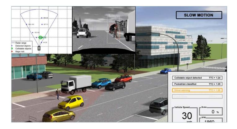
high-frequency electromagnetic radar models and physics-based camera models for sensor technology development. Thermal analyses tools are also available to engineers to support sensor design and sensor integration in the vehicle.
