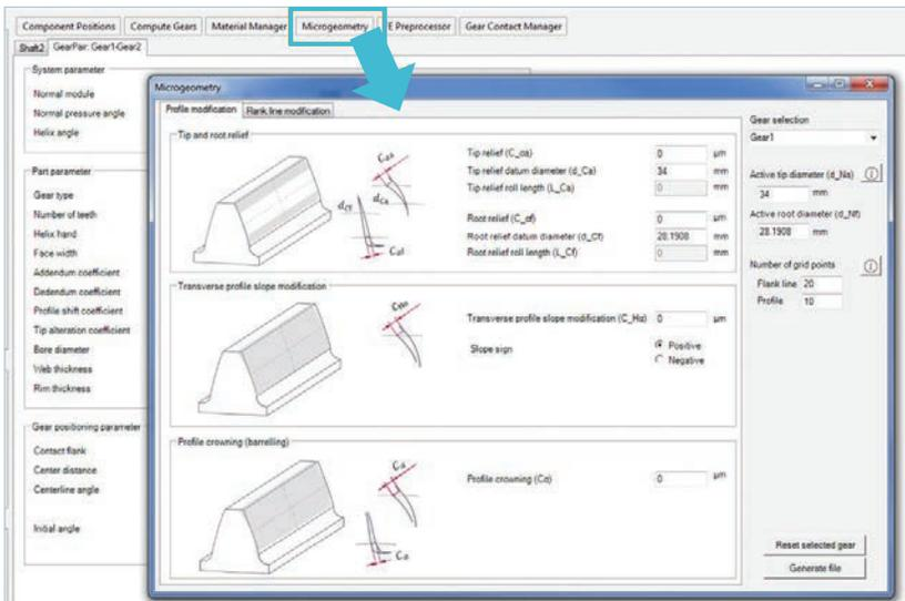
Figure 4: Microgeometry creation.
