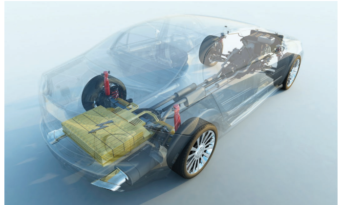
Figure 1. Hybrid electric vehicles have both electric and traditional powertrains to power various systems within the vehicle.
