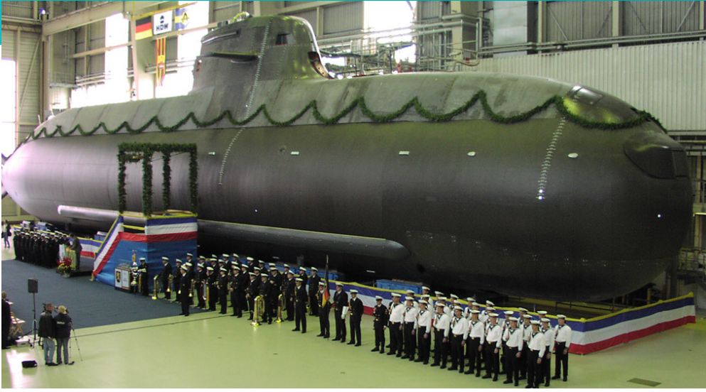
This shows the dividing line between where composites (top) and metal (the hull) have been used on this class 214 submarine. HDW is using Fibersim to design and manufacture the complete upper deck, keel covers, tower sail fairings, propeller blades and rudders.
