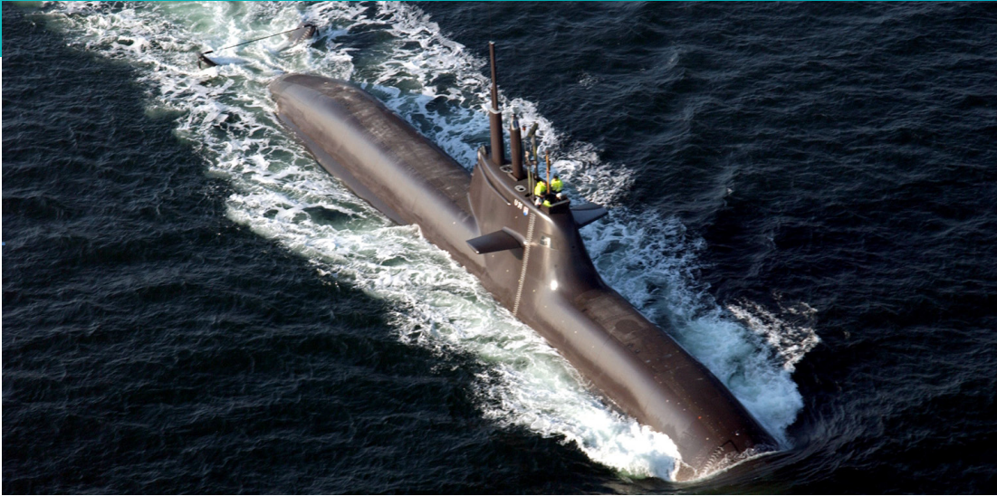
"When a Class 212A or a class 214 submarine are surfaced, everything that you see is made of composites," says Marc Tillmanns, lead composites engineer at HDW. The use of composite materials results in a sleeker silhouette and reduced wake.
