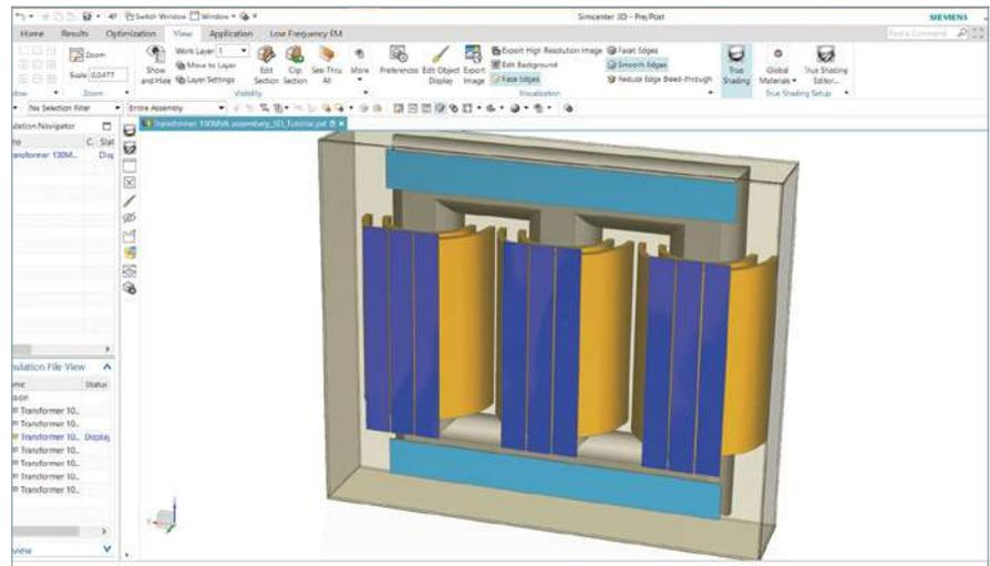
Figure 1: 100 MVA Power Transformer assembly in Simcenter 3D
