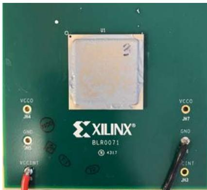
Figure 1: Xilinx Package mounted on JEDEC 2S2P PCB
