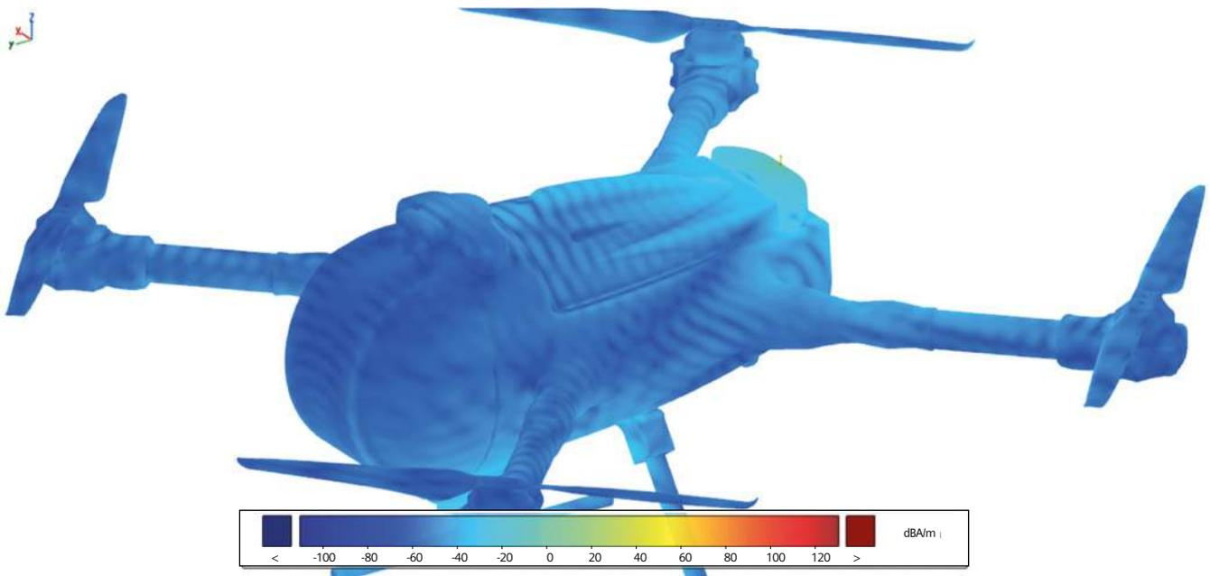
Figure 3: Induced Currents on a Colibri Drone
