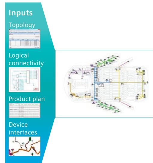
Figure 3: The four primary inputs to a generative design flow include harness topology, logical connectivity, product requirements, and device interfaces.
