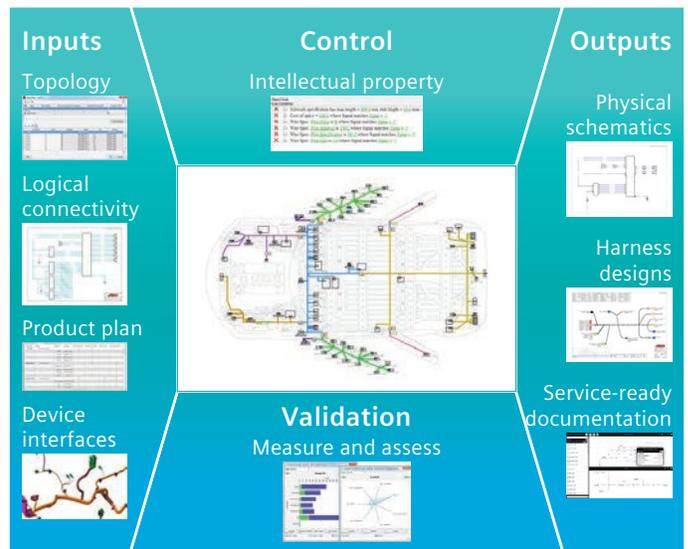
Figure 5: Generative design uses rules-based automation to generate outputs, and can create metrics to assess designs and change impacts.
