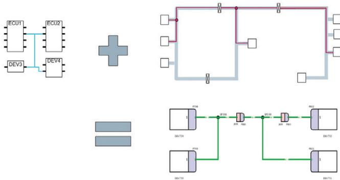
Figure 1: Generative design combines system connectivity definitions with physical harness layouts to synthesize wiring designs.
