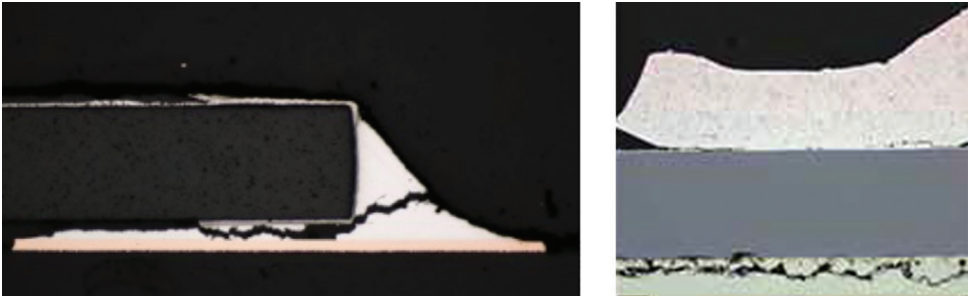
Figure 2: Example of solder cracking and wire bonding crack.
