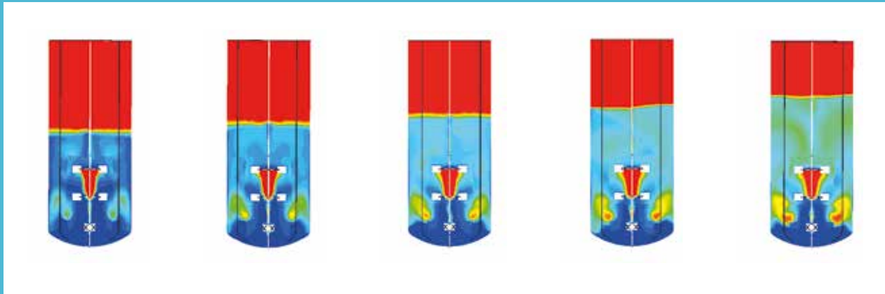
Figure 4: Mixer model showing the effects of increasing gas injection rate using Simcenter STAR-CCM+.
