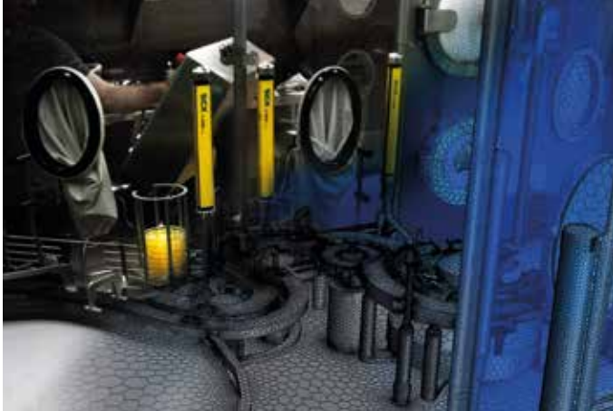
Figure 3: Hexahedral mesh of vials conveyor.
