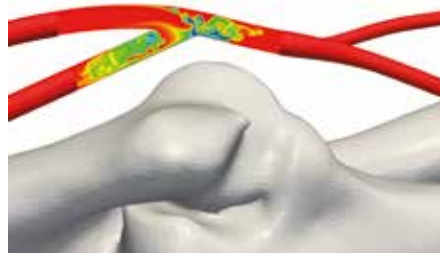
Figure 5: Concentration of a passive scalar, advected with blood flow, on a centerline plane section in the AVF.
