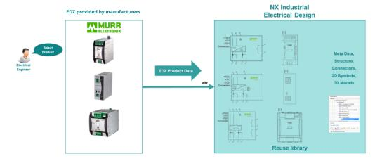
You can use the EPLAN EDZ format to import product data into the product library, including properties, structure, connectors and 2D symbols. The 2D symbols for the different representations (multi-line electrical schematic, 2D cabinet layout) are imported. The EDZ import extension significantly reduces the effort needed to create new products and improve access to vendor-neutral formats.
