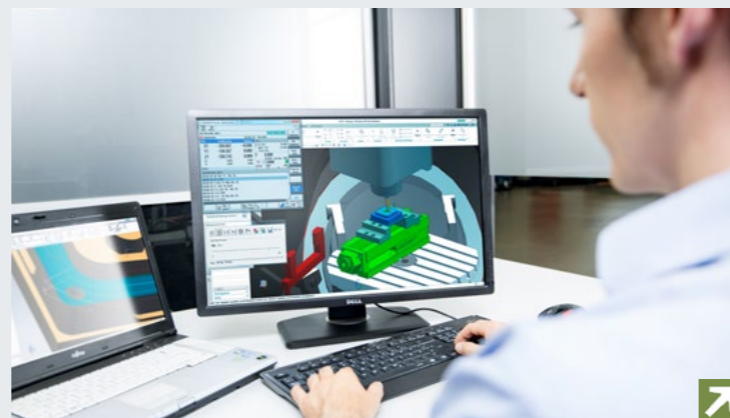
Virtual NC Kernel (VNCK): Enabling virtual tests in parallel with real op- eration using the original SINUMERIK software
