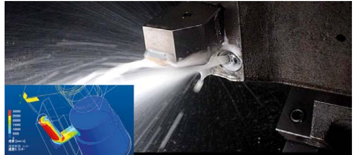
Mitsubishi materials corporation uses Simcenter FLOEFD to design liquid-cooled nozzles for cutting tools
