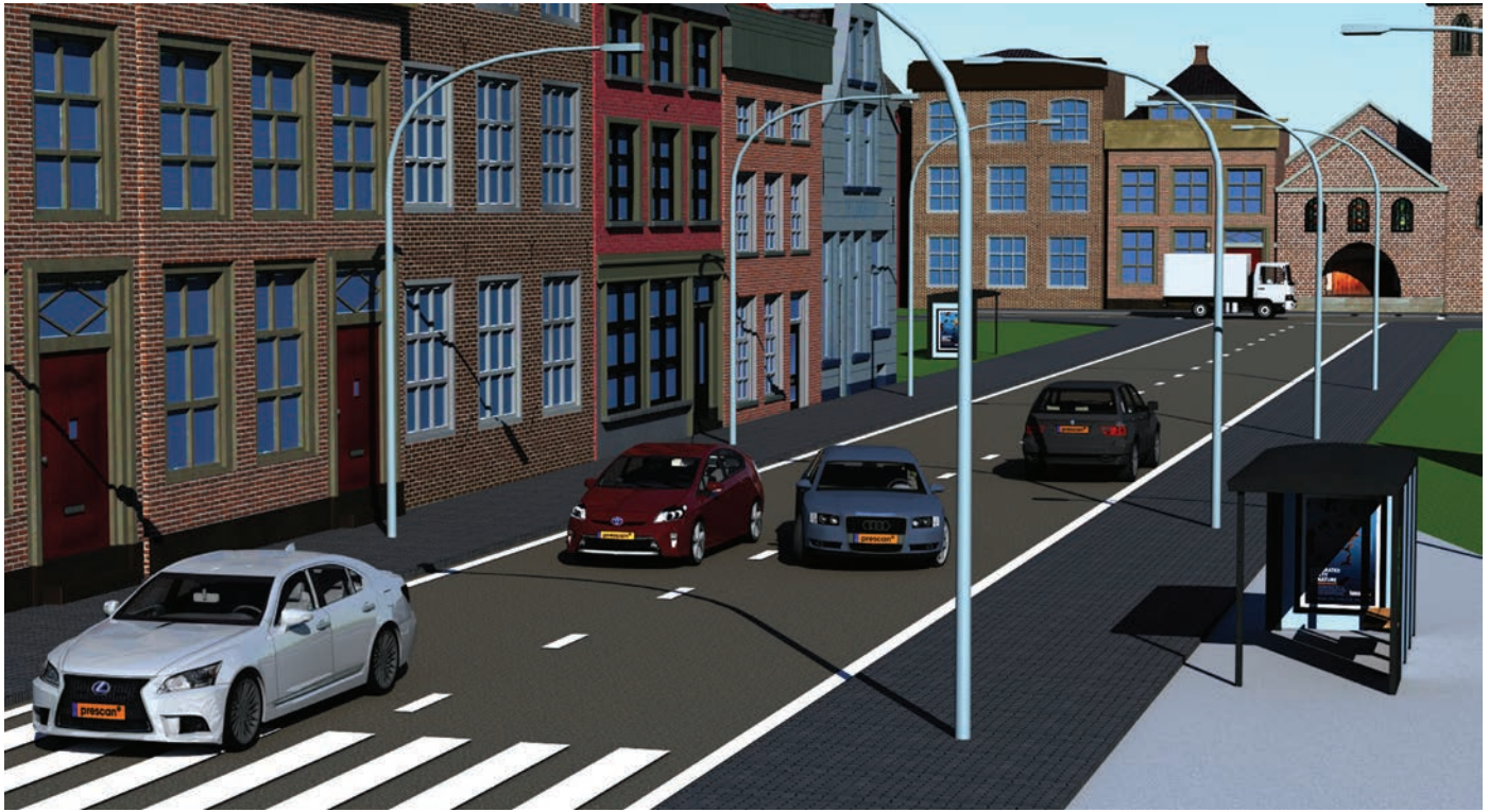
Figure 4: PreScan screenshot; tool uses ray tracing to model a one-lane-change evasive maneuver.
