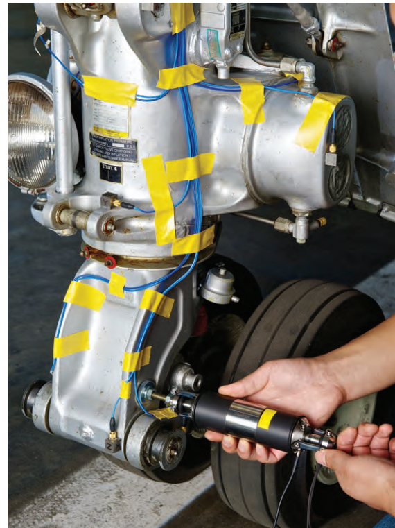
Simcenter engineering can help you mitigate problems related to shimmy. We help you trace its root cause and determine design alternatives. Image courtesy of Belgian Defense.
