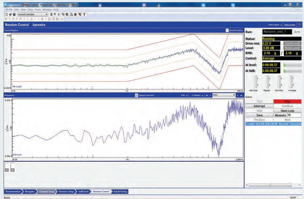
Simcenter Testlab Dynamic Environmental Testing helps to qualify aerospace components reproducing vibration loads in a safe and accurate manner. Image courtesy of SABCA.
