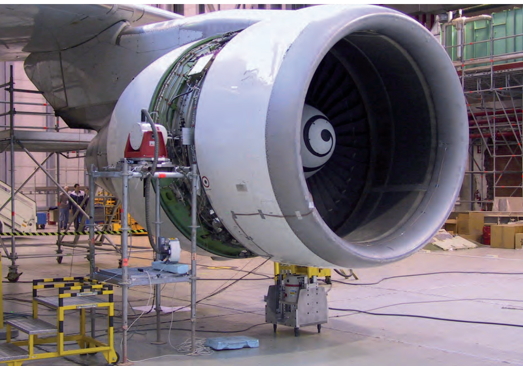
Understanding engine pylon non-linearities to prove compliance with sustained engine imbalance certification requirements. Image courtesy of Airbus Defense and Space.
