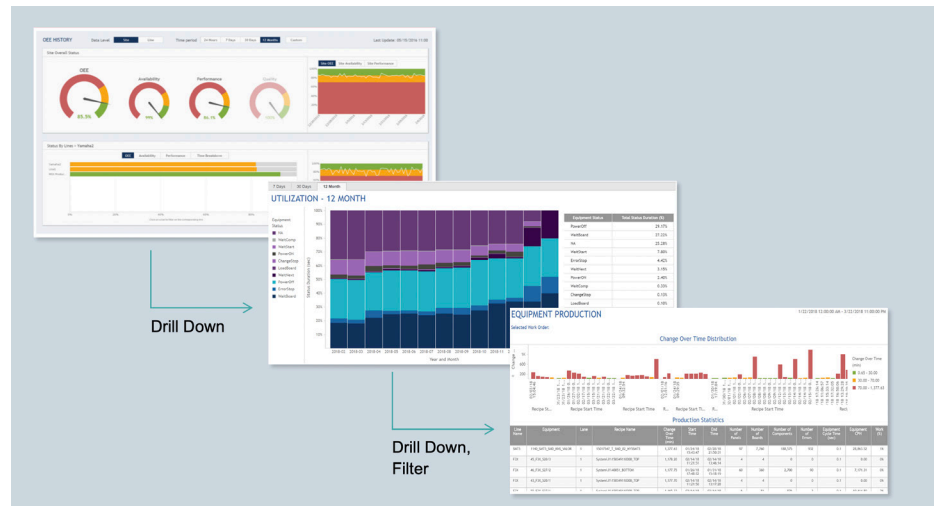
Figure 2: Opcenter Intelligence Electronics is a big-data, business-intelligence analytic platform for high-performance manufacturing. It provides greater visibility into equipment, products and supply-chain performance, easily identifying and monitoring production and supplier issues, preventing costly recalls, spotting emerging trends and solving quality problems faster than ever before.
