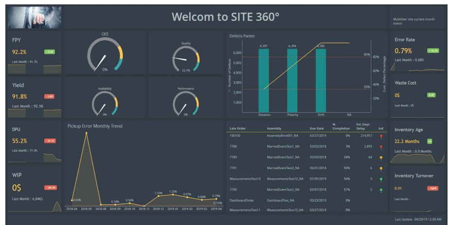
Figure 1: View and drill down to access real-time smart data, including enterprise resource data (ERP) data integrated with manufacturing KPIs such as yield, WIP value, inventory turnover and waste costs.
