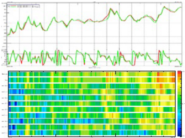
Figure 17: On-board validation in target t1 for order 90. Top: Comparison of measured target (red) and predicted target (green) using blocked forces determined in-situ from the original assembly. Bottom: predicted contributions
