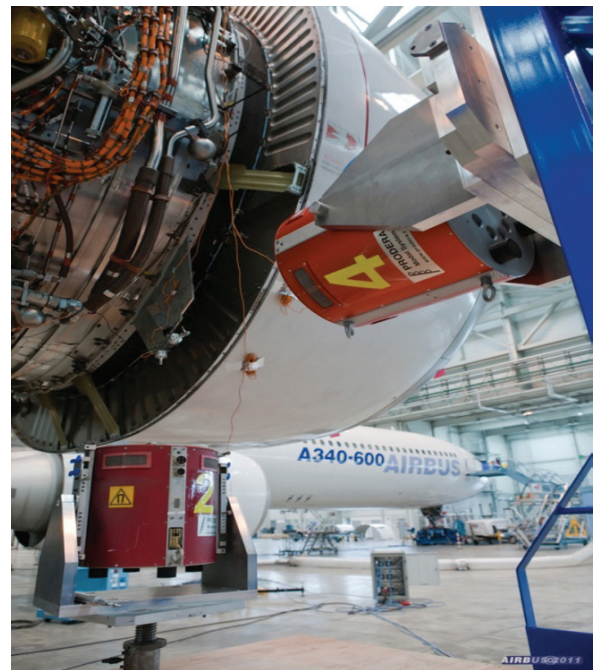
Lateral and vertical exciters placed on the aircraft engine during the certification of the A340-600 (images courtesy of Airbus, Onera and DLR).
