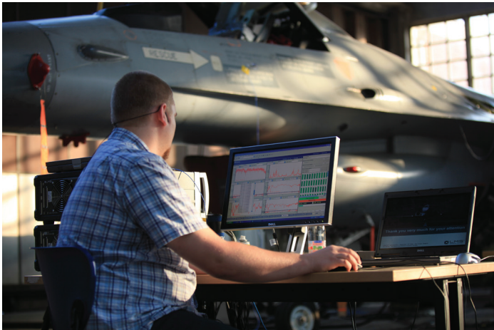
Ground vibration testing: modal test on the full aircraft structure as part of the certification process.
