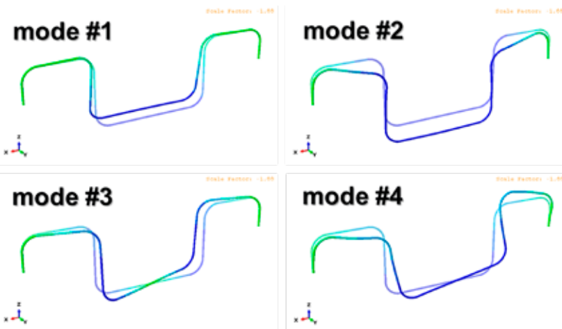
Figure 4: First four natural modes of the jumper
