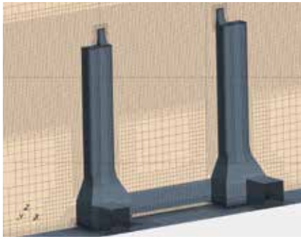
Figure 6: Trimmed mesh on GBS (left) and wave profile around GBS (right)
