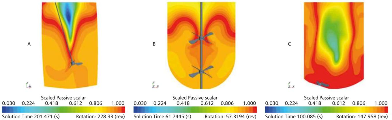
Figure 4: Comparing CFD simulations at full scale (at 95 percent volume uniformity) for each platform option, showing more homogeneous mixing in platform B
