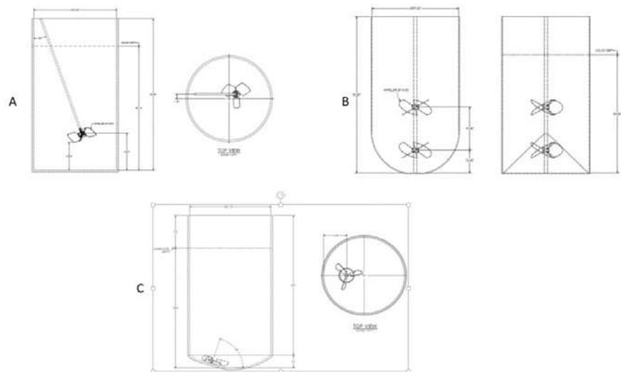
Figure 3: Platform options for bioreactor performance evaluation
