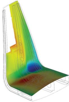
In addition to modeling, Simcenter 3D can help you validate your draping simulation to help you understand how the fibers will be oriented on your part.
