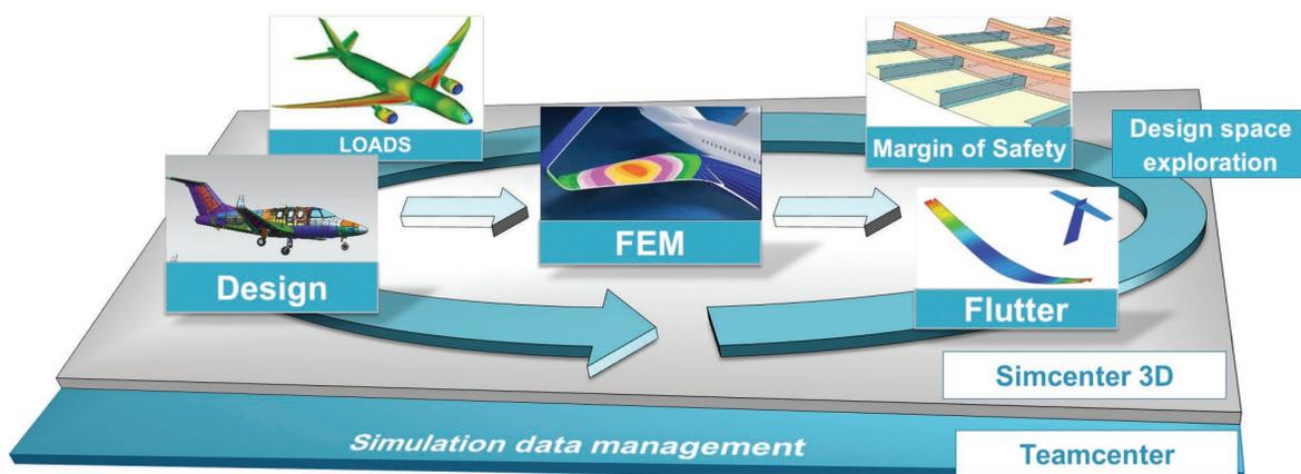
Simcenter 3D provides out-of-the-box load case enveloping capabilities that can help you quickly find the most critical loads for a component or an entire assembly.
