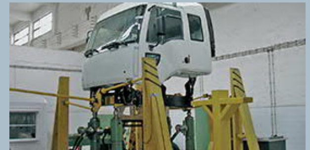
Cabin rig test to represent 1.2 million kilometers
