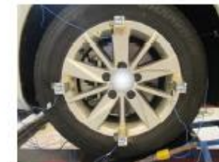
wheel instrumentation for NVH tire characterization
