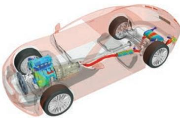
Figure 6: Heat flux from engine surface to ambient environment at 240 KPH and 135 kW.
