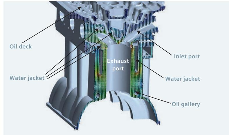
Figure 5: Heat flux vectors in the engine structure.
