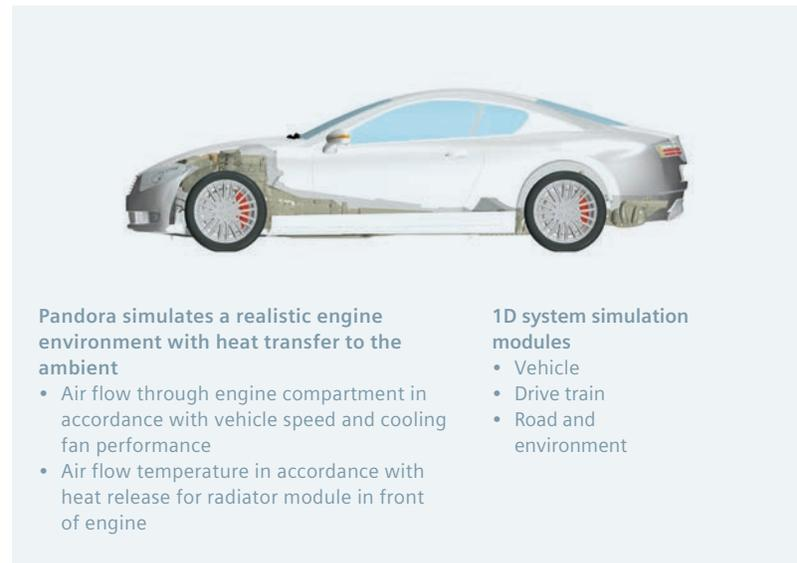
Figure 3: Pandora is a virtual concept car with underhood and full-vehicle environment that was modeled with Simcenter STAR-CCM+ to simulate engine thermal performance with heat transfer to the ambient environment.
