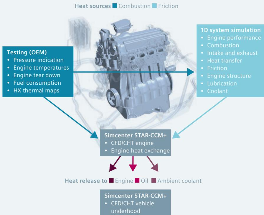
Figure 1: InDesA's approach to engine and vehicle underhood thermal simulation.
