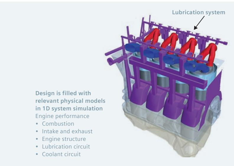
Figure 2: The virtual engine is brought to life with data from 1D simulation.
