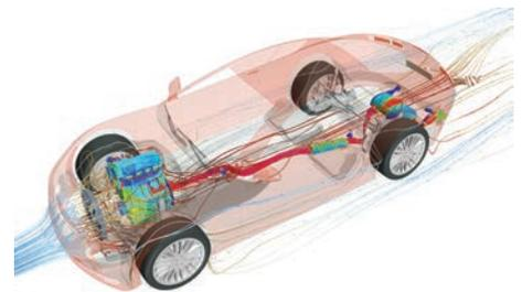
Figure 8: Streamlines through engine compartment for 240 KPH at 135 kW.
