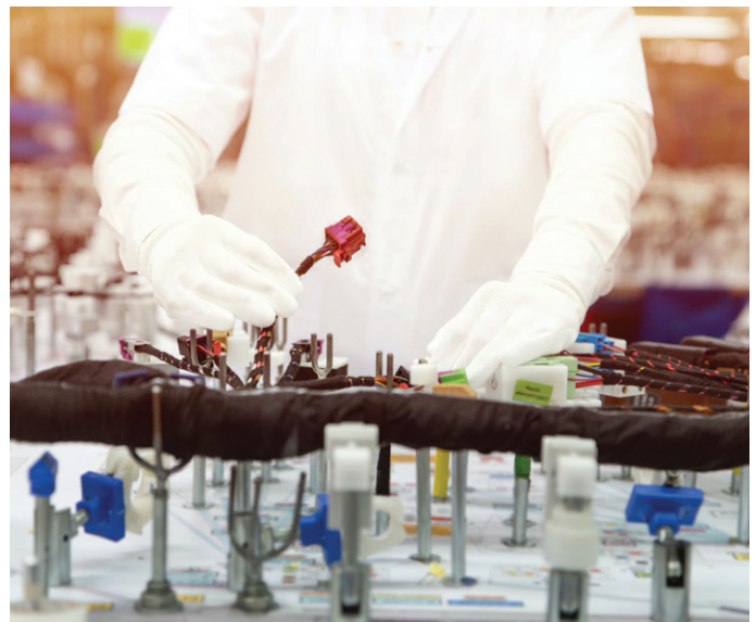
Figure 2. Harness rework allows suppliers to resolve issues in as-produced harnesses, adapt to changing customer orders and more, but it is very costly.
