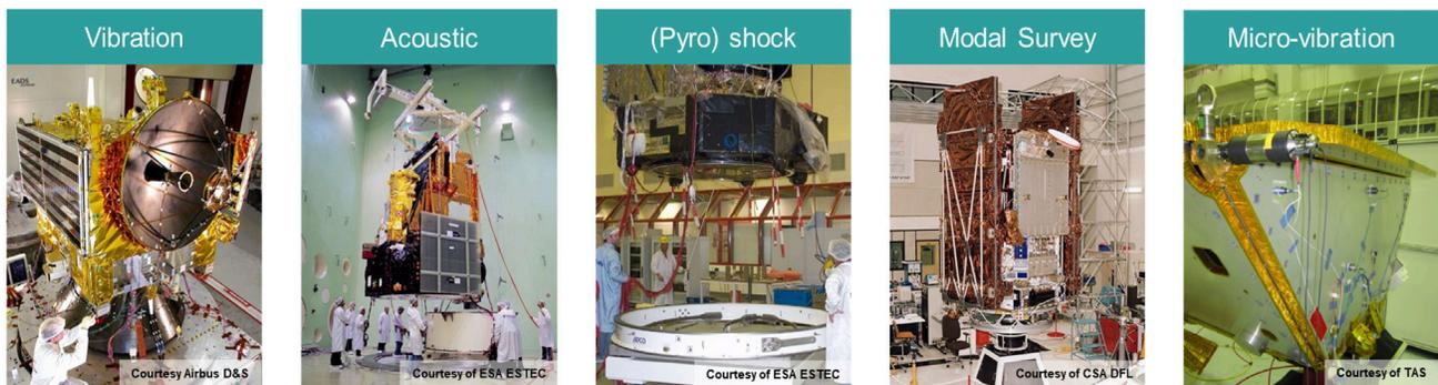
Figure 3. Space hardware validation involves different types of testing: mechanical qualification, modal survey and micro-vibration testing.
