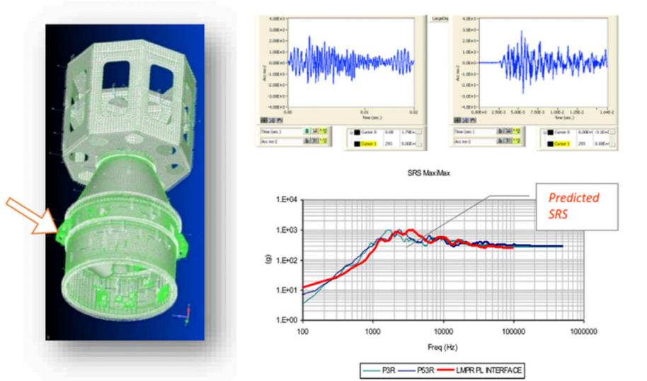
Figure 14. SEA prediction of VEGA launch vehicle upper part. Top-left: predicted and measured acceleration time history on payload interface. Bottom: predicted and measured SRS on payload interface.
