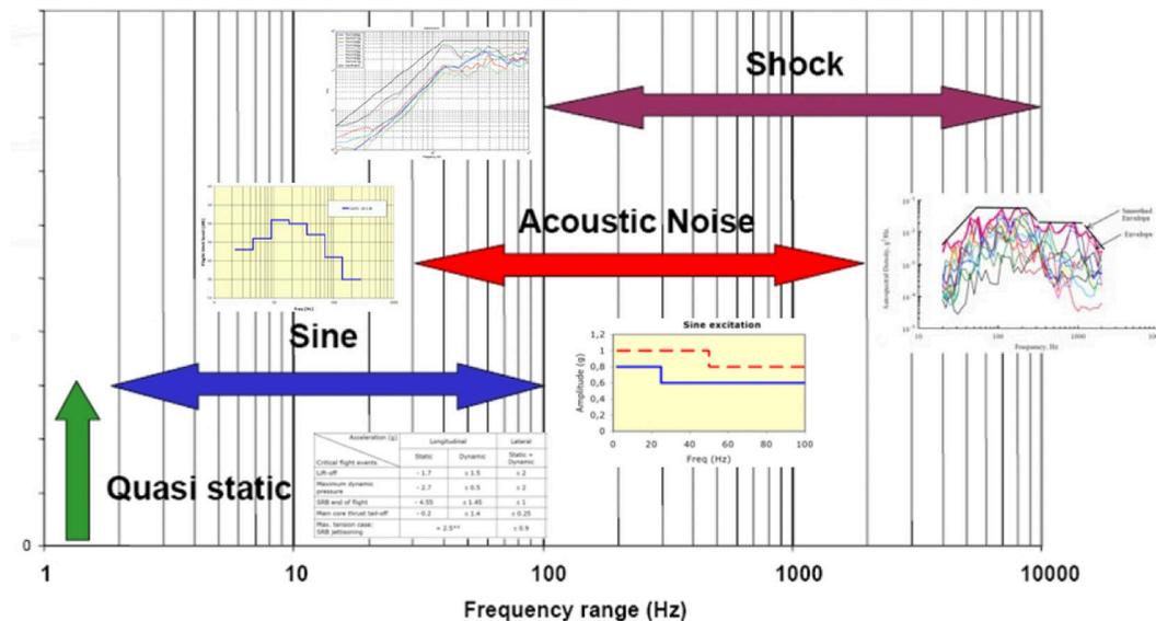
Figure 2. Vibration environments and corresponding frequency ranges.
