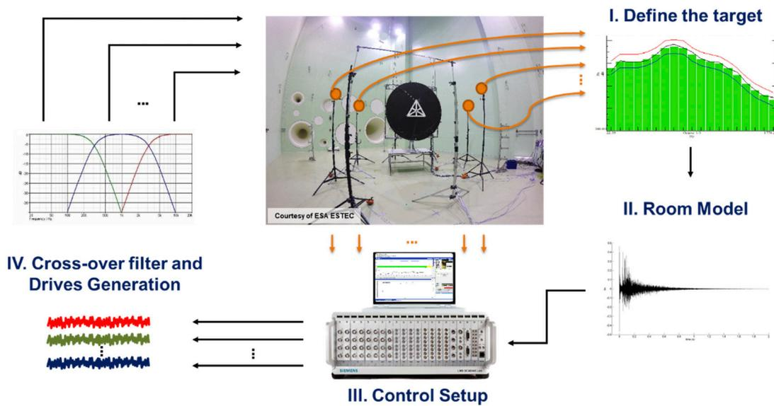
Figure 10. Schematic representation of an acoustic control system.
