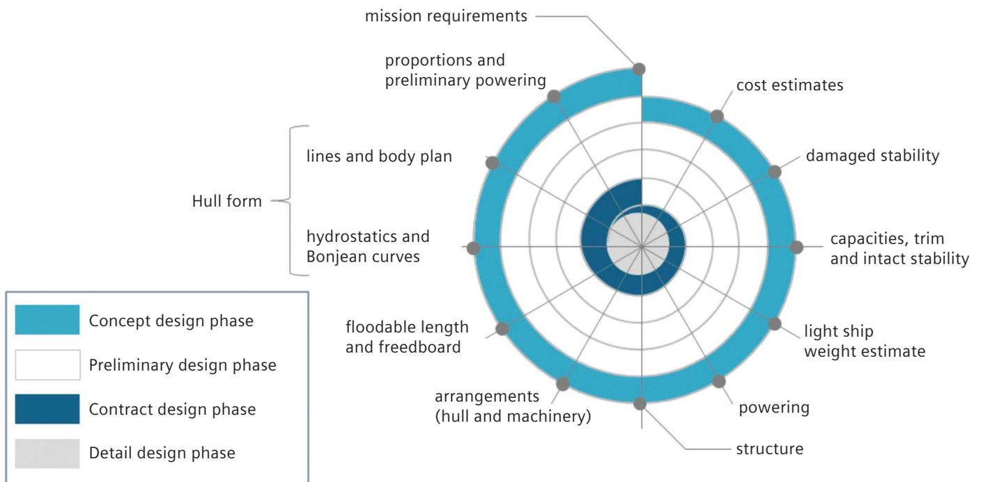
Figure 2: Pictured is the vessel design spiral. Each refinement of the vessel design passes through a sequence of requirement assessments until the final design is reached.
