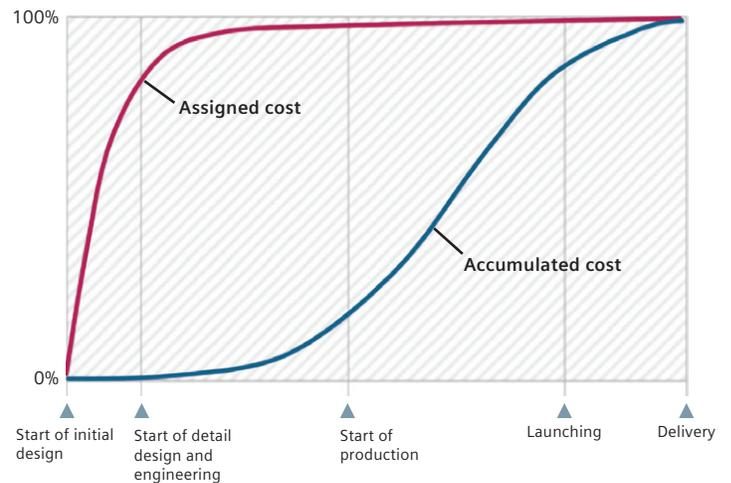
Figure 1: Typical cost build-up for a ship based on work by Fisher and Holbach, 2011.<sup>1</sup> Approximately 85 percent of the final vessel cost is determined during the early design phase.
