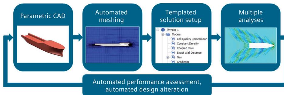
Figure 4: Automated simulation process. Any changes in CAD can be rapidly assessed and the user isn't required to set up models.
