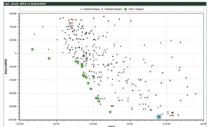
Figure 7: Overview of all investigated designs, with relative CAPEX and OPEX. There are a range of feasible designs (green) that meet the design constraints.
