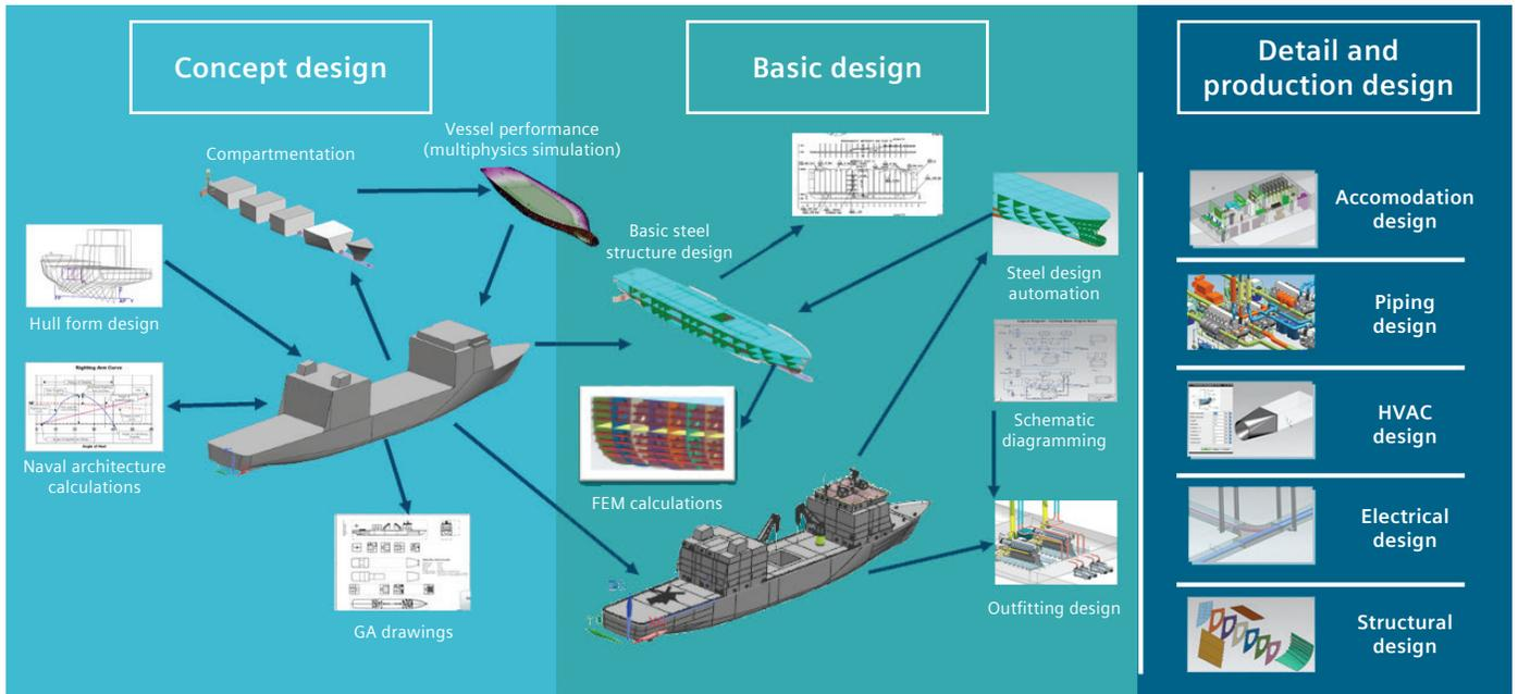
Figure 3: Integrated design environment, with communication both within and between design stages.
