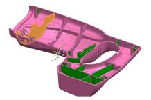
product design and identify key features such as bends, embossing and sheet metal thickness that influence the manufacturing of stamping tools. Once the features are analyzed and identified, the information is transferred to Teamcenter tool costing software to estimate manufacturing costs.
