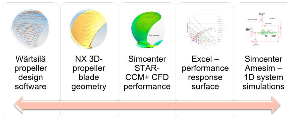
*The simulation process at Wärtsilä to design marine propellers.*
