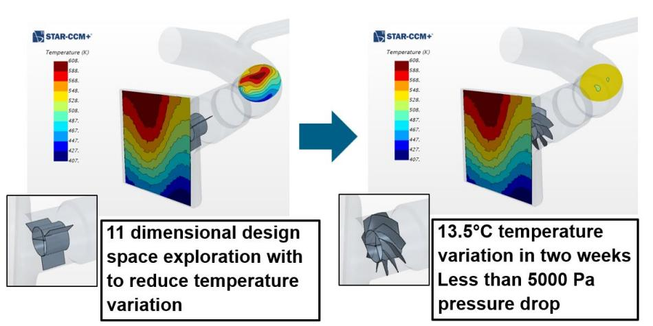
*Baseline and optimized design of aircraft bleed-air system on an Airbus A320.*
