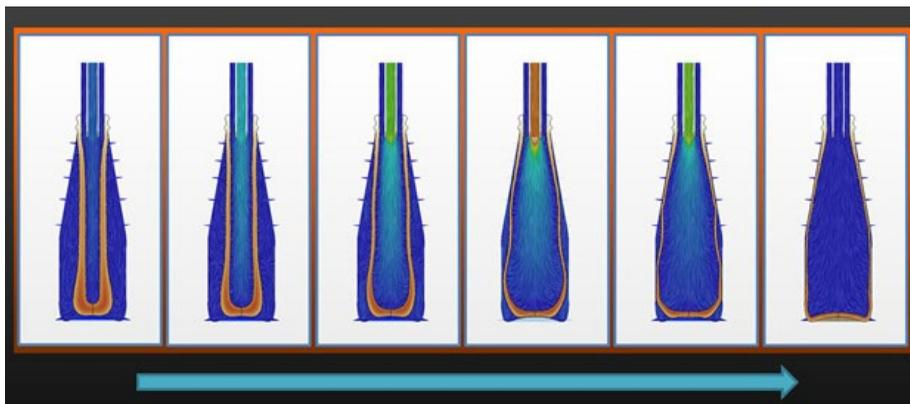
*Bottero use simulation not only help the bottle design, but engineers were also able to decrease the bottle mass. Image courtesy of Bottero/Siemens Digital Industries Software.*
