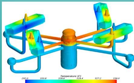
One of the largest nuclear CFD simulations from OKB Gidropress using Simcenter STAR-CCM+.
