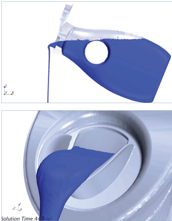
Figure 7: Simcenter STAR-CCM+ simulation showing the pouring process from a typical laundry detergent pack with a close-up of the nozzle design.
