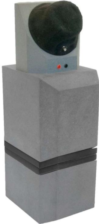
The unique properties of this low-mid frequency source include, human body diffraction simulation, time stable sensor sensitivity and high noise levels. These features make this device extremely accurate and efficient for the analysis of transport vehicles like cars, vans, trucks, busses, trains and aircraft.
